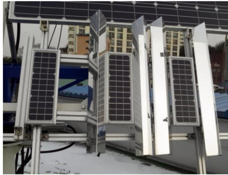
Figure 6. Solar Concentrator Module 7.2W
