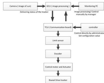
**Figure 5. The Overall System Operation Environment**
