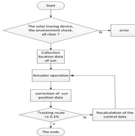
**Figure 1. Basic Operation Flow Chart of Solar Tracking System**
