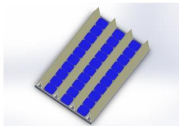
**Figure 4. The Estimated Structure Diagram of Solar Concentrator Module Equipped with A Reflection Plate**
