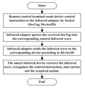
Figure 3. The Communication Process between Remote Control Terminal and Infrared Adapter
