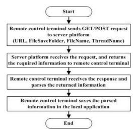
Figure 2. The Communication Process between Remote Control Terminal and Server Platform
