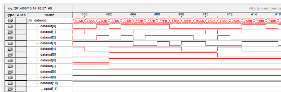
Figure 10. A/D Sampling Signal Captured By Signal tap II
