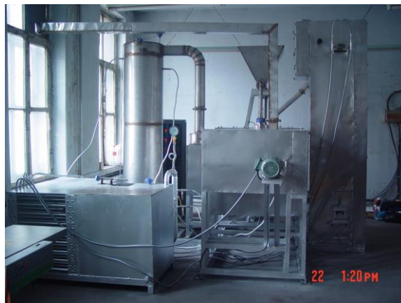
Figure 2. The Real Heating Furnace with Circulating Air-duct
