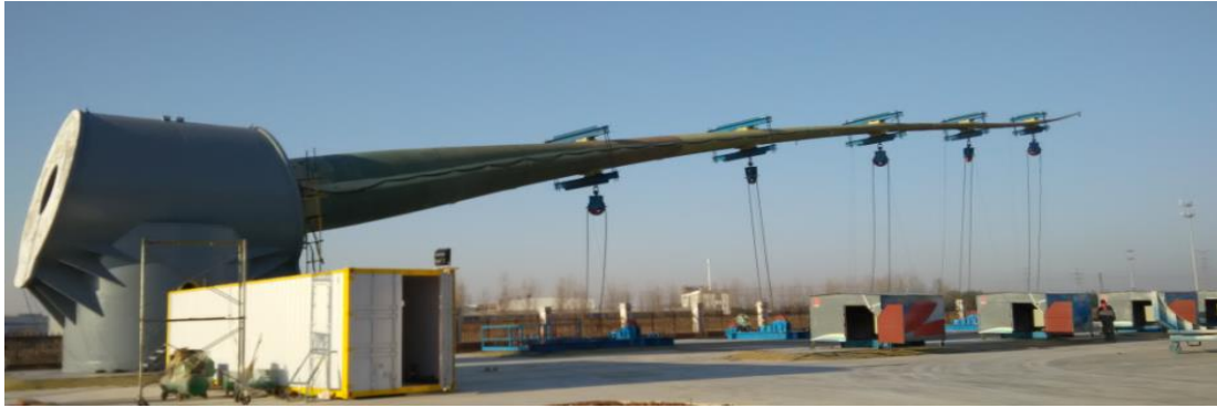
Figure 7. In-site Test of Static Loading
