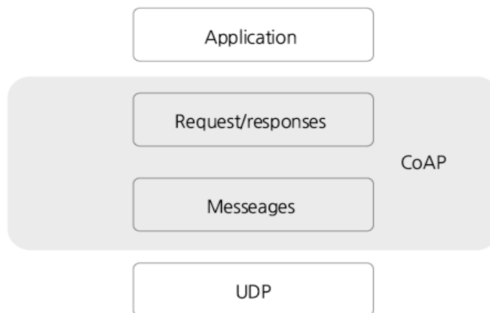
Figure 2. CoAP Protocol Stack
