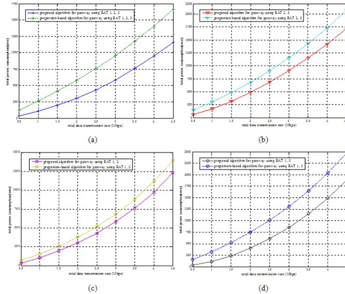
**Figure 3. Total Power Consumptions Using the Two Algorithms**
