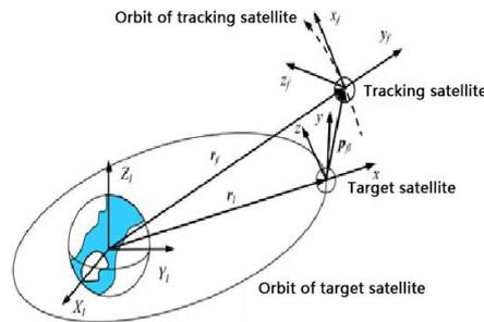
**Figure 2. Definition of Coordinate System**
