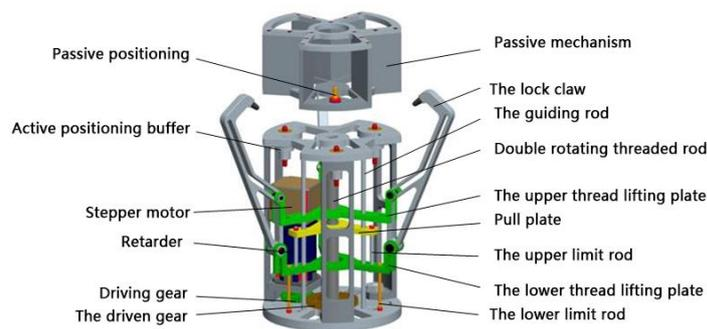
**Figure 1. Structure of the End Executor**
