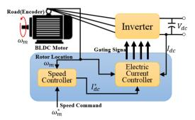
Figure 4. Speed Controller System Using Electric Current Controller
