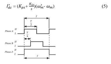
Figure 5. Phases A, B, Z Using in the Incremental Encoder
