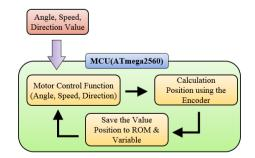
Figure 6. The Motor Controller Operating
