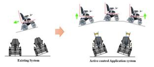
Figure 2. Maintain Seat Balance of Electric Wheelchair System
