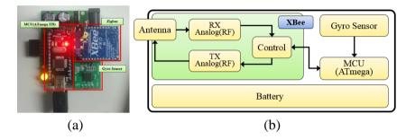
Figure 9. (a) The Sensor Module System for Identifying Terrain (b) Functional Structure
