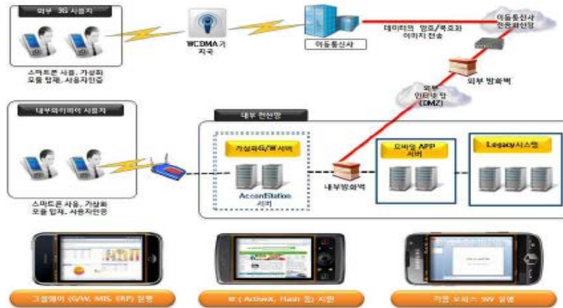
Figure 2. Cloud-based Mobile Office Service
