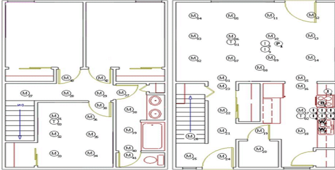
Figure 1. Sensors in a Smart Home, Monitor Motion (M), Temperature (T), Water (W), Burner (B), Phone (P), and Item Use (I)
