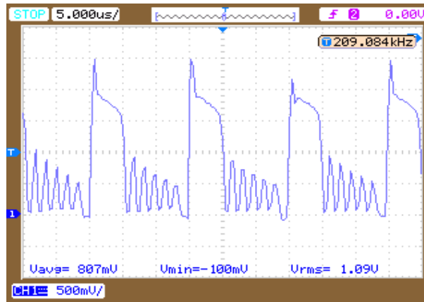
Figure 16. The Voltage Signal of FB Pin (4.7Ω)
