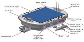
**Figure 5. Sensor Robot**
