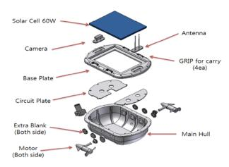
Figure 6. Robot Platform Internal Structure
