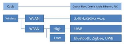
Figure 1. Wireless Data Transfer Technology
