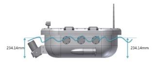
Figure 6. Line that the Sensor Robot Sinks to the Water
