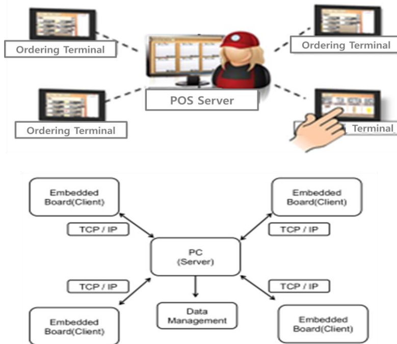
Figure 1. Overview of Unmanned Ordering and Payment System and its Hardware Structure using Embedded Devices
