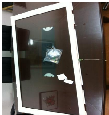
Figure 2. Rectangular antenna and distributed capacitor between coils
