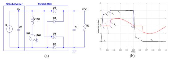
Figure 5. Parallel synchronized switch harvesting on inductor interface
