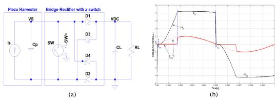
Figure 3. Standard interface with a switch: (a) circuit schematic and (b) waveforms
