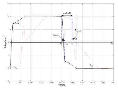
Figure 7. The definition of switch triggering offset and on-time deviation: p-SSHI
