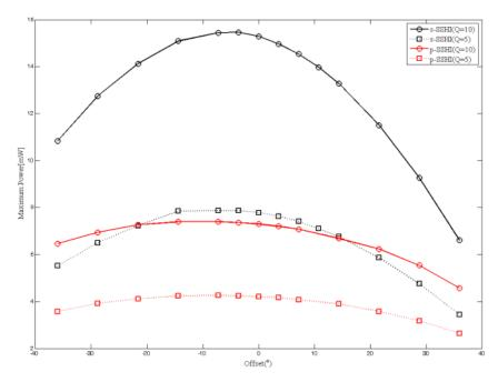
Figure 9. The harvested power as a function of the switch triggering offset
