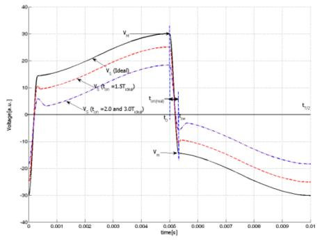
Figure 11. The voltage waveform depending on the on-time duration deviation in s-SSHI
