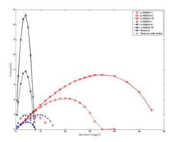
Figure 4. The comparison of power harvested by different interface circuits
