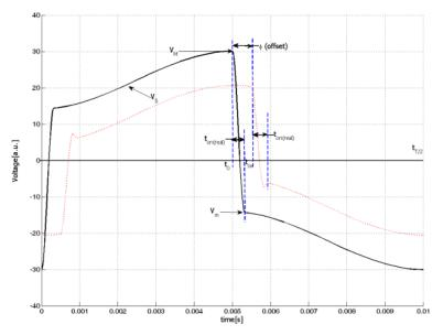
Figure 8. The definition of switch triggering offset and on-time deviation: s-SSHI
