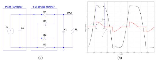
Figure 2. Standard interface: (a) circuit schematic and (b) waveforms
