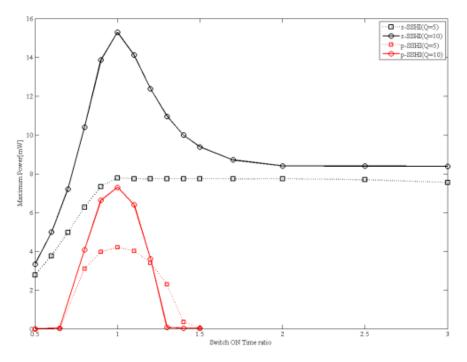
Figure 10. Harvested power as a function of the switch on time duration deviation
