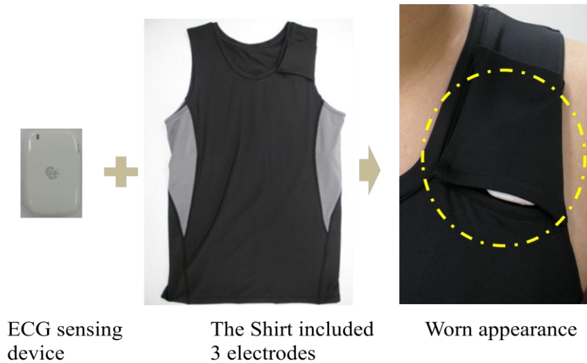
Figure 6. The Proposed Wearable ECG Hardware
