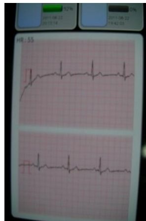
Figure 7. The ECG Signal Graph on the Smartphone
