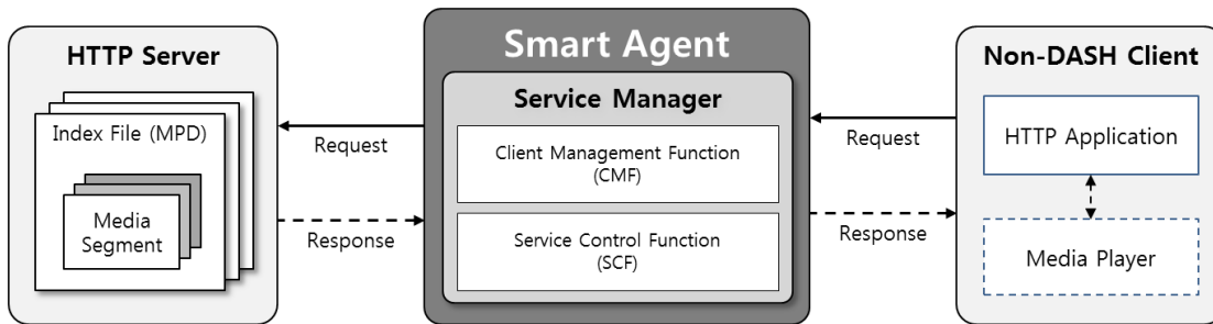
Figure 2. The Structure of the Existing Proxy Server
