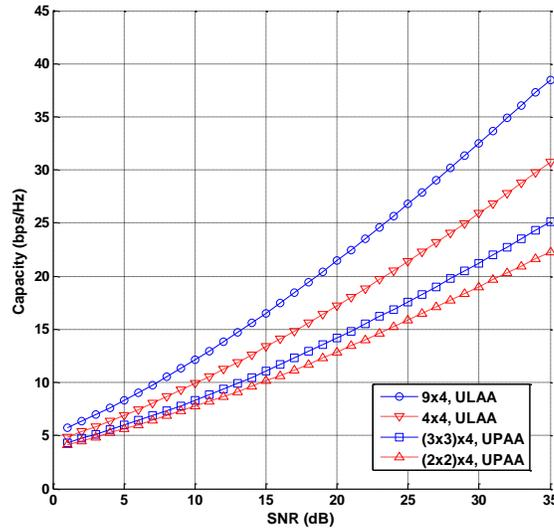
**Figure 4. Capacity of the Different Antenna Structures with Mean 8° AS**
