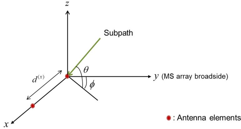
**Figure 2. ULAA with 3D Subpath**
