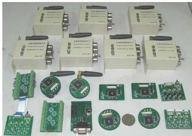
Figure 2. The Picture of the Designed Wireless Strain Node, PZT Node, Station Node and Shock-proof Encapsulation
