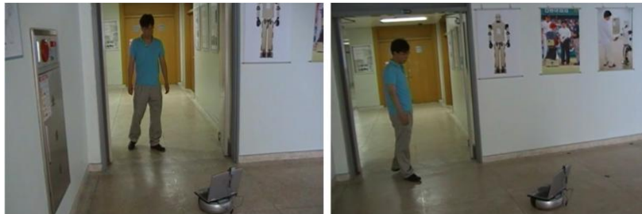
Figure 3. Experiment of a Human-Following Services using a Mobile Robot, X-Bot
