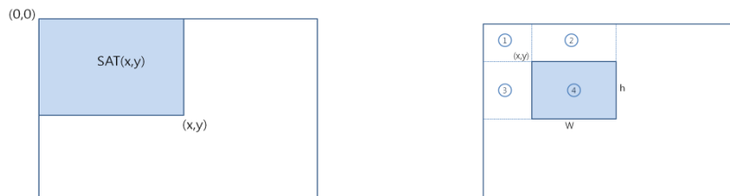
(a) SAT (b) sum of pixels in the rectangle Figure3. Integral image of the rectangle
