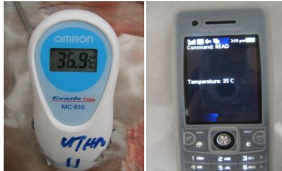
Figure 6: Comparison Temperature Reading of Thermometer and Temperature Sensor
