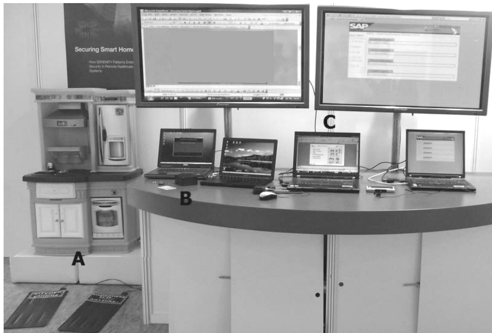
Figure 4. Prototype Demonstration: A) Smart Kitchen and sensitive rugs; B) oxymeter; C) client PCs
