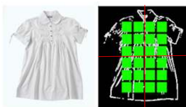
Figure 3. Input garment image and the black-white edge image. Those green blocks are the grid set for recording locality.
