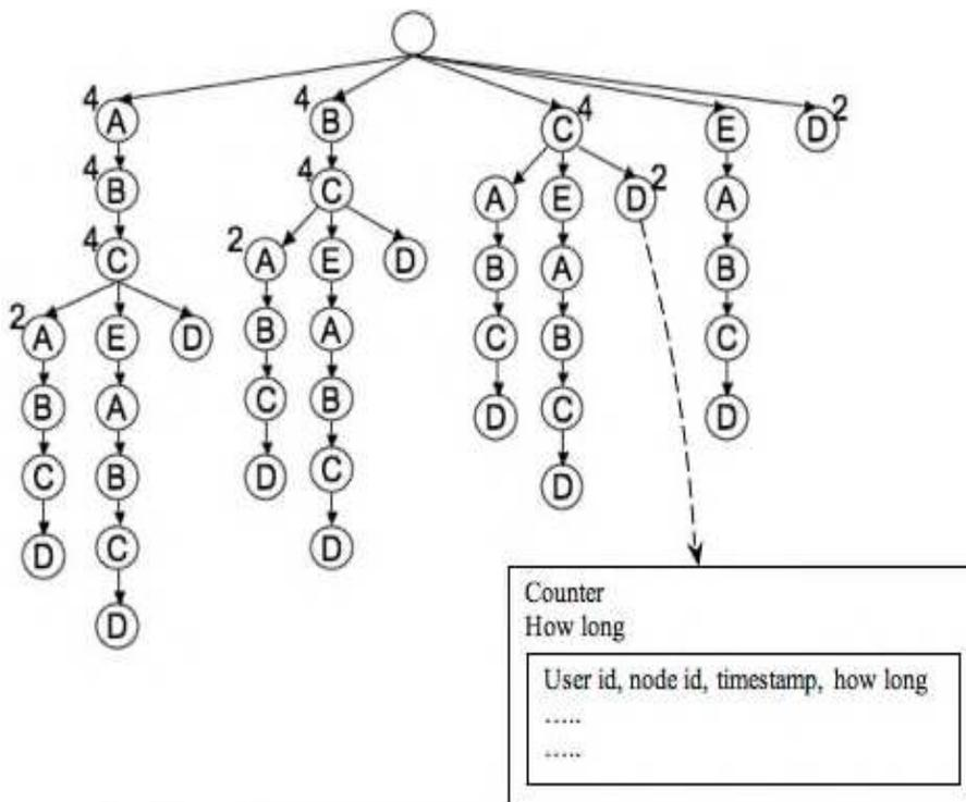
**Fig.1** - Suffix tree containing two trails, namely ABCABCD and ABCEABCD. Each letter represents a wireless sensor nodes with which at least one robot has interacted with. Each node is also associated with additional metadata used to answer and rank significant trail queries.
