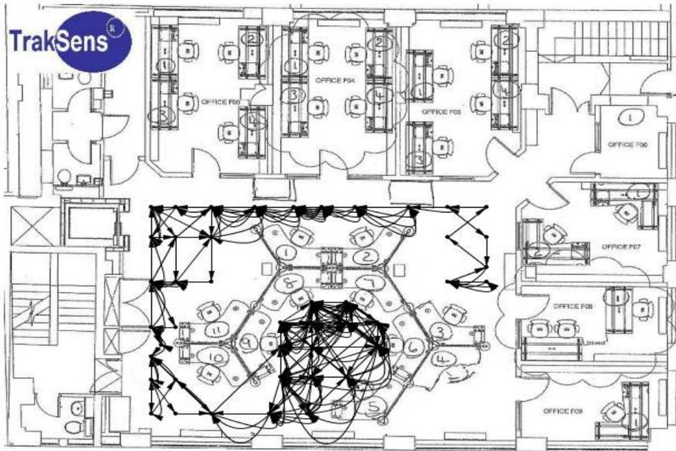
**Fig. 6** – This figure shows the trails followed by the robotic cleaner – represented by the arcs and arrows. It is clear that within the time frame given (one hour) many spots within this space were not covered at all.
