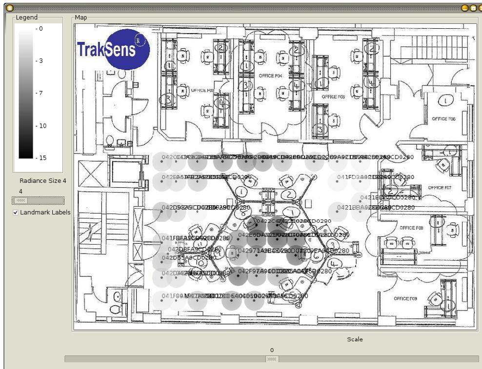
**Fig. 5** – Screenshot of the GUI of our system – the office plan where the robotic cleaner was deployed is shown together with hotspots of activity (represented by circles). Darker circle colors represent landmarks that were visited more often than others.
