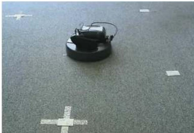
**Fig. 4** – iRobot Roomba Robotic Cleaner with Surrogate Device mounted on top of it. Also visible in the picture, are the RFID tags attached to the floor, forming a proximity grid.
