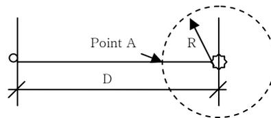
The distance from the sink to the centre of the physical signal field is  $D$ ,  $D > R$ . For each node, the cost value  $V_c = c_2 * d$ , in which  $d$  is the distance to the sink, and  $c_2$  is a constant,  $c_2 > 0$ .
