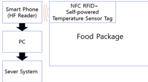
Figure 2. Block diagram of next generation temperature history system.
