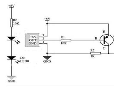
Figure 5. Laser Detection Module Hardware Circuit
