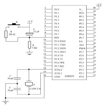
Figure 2. Single Chip Microcomputer Minimum System
