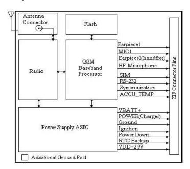
Figure 3. TC35 Function Block Diagram
