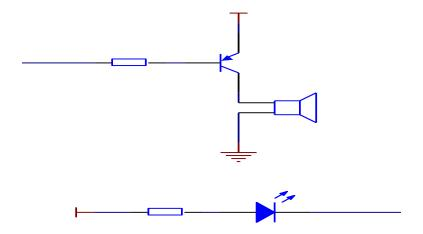
Figure 6. Acousto-optic Alarm Circuit
