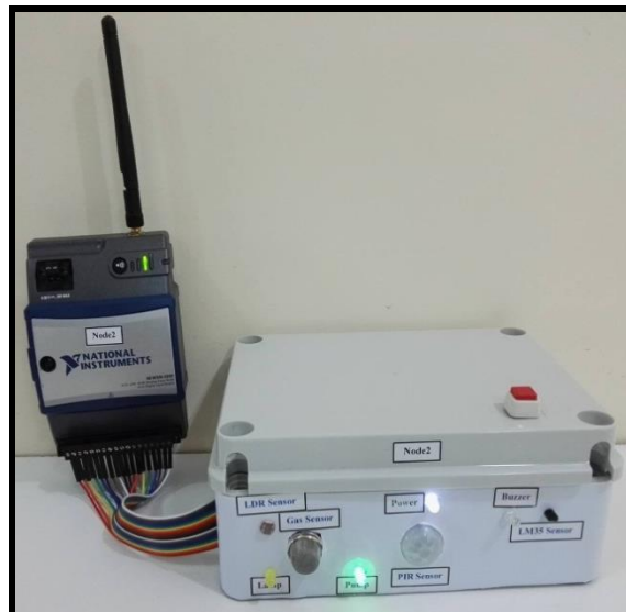
Figure 14. Indication LED to Operate Firefighting Pump
