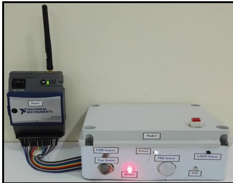
Figure 8. Indication LED to Operate Heater
