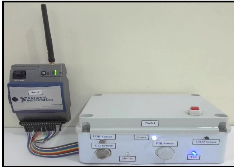
Figure 6. Indication LED to Operate Fan
