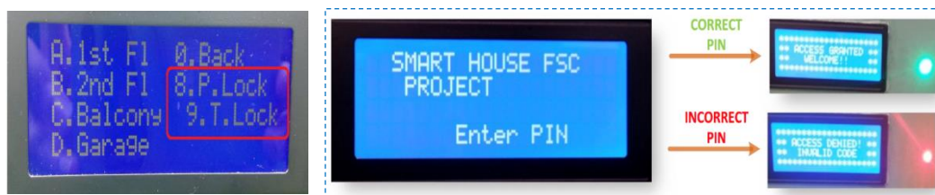
Figure 10. Security Levels and Pin for the House
