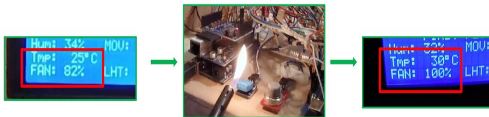
Figure 30. Testing the Fan's Speed Using a Lighter
