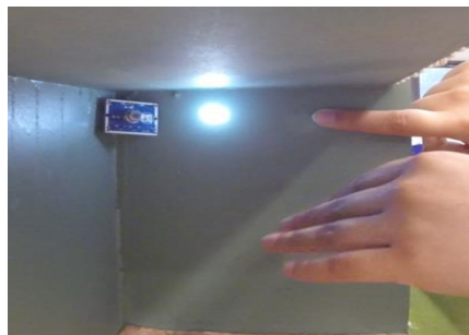
Figure 33. Testing the Backyard Light Subsystem
