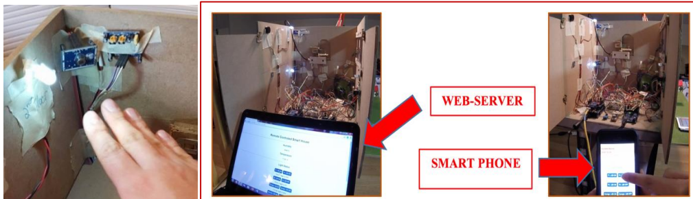
Figure 29. Testing the Light Control Subsystem Manually and Remotely
