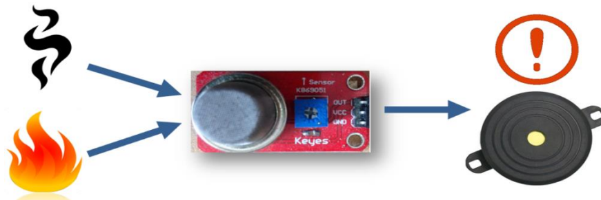
Figure 3. Safety Subsystem - Fire and Smoke Detector
