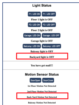
Figure 14. Backyard Light Control using Web-server
