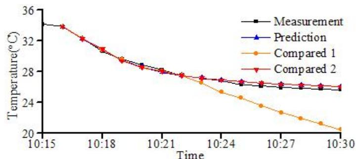
**Figure 5. Prediction of Greenhouse Air Temperature in the Mechanical Ventilation Sub-State**
