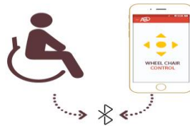
Figure 11. The Wheelchair is Fitted with Electric Motor and Bluetooth module. This Motor can be Controlled by the User's Smart-Phone via Bluetooth.
