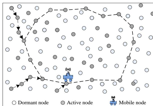
**Figure 1. Data Collection with Mobile Sink in Low-duty-cycle Sensor Networks**
