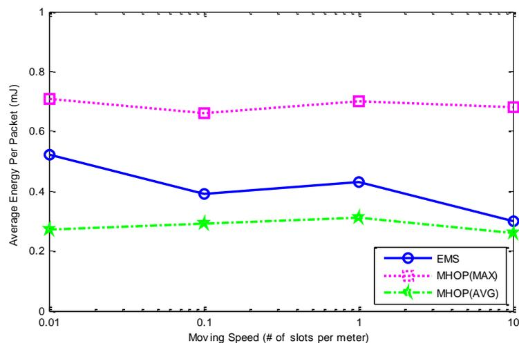
**Figure 10. Energy Consumption vs. Moving Speed**
