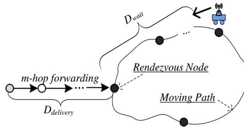
**Figure 4. Delay Modeling in Multi-hop Data Forwarding**
