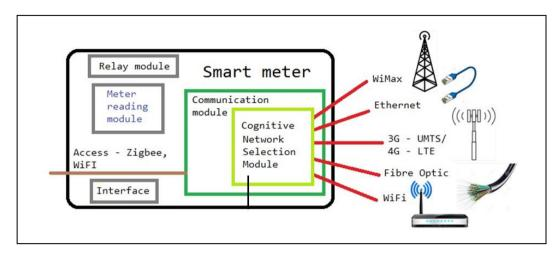
Figure 3. Proposed Multiple Backhaul Network Connection Smart Meter with Self-Switching Capability
