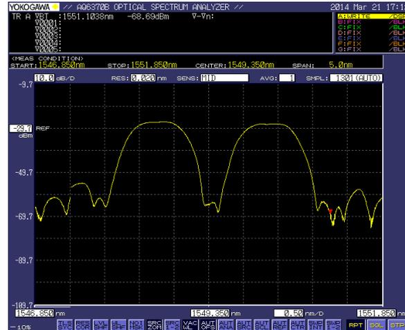
**Figure 7. AWG Dual Channel Transmission Spectrum**
