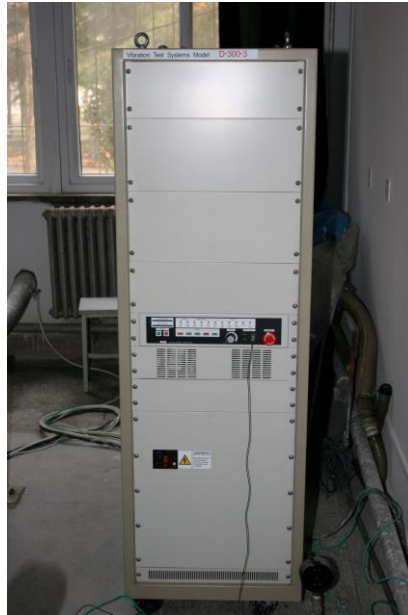
Figure 2. Photograph of SA1-3 Power Amplifier
