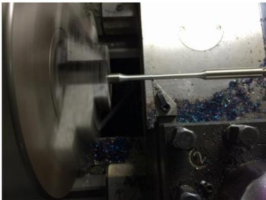
**Figure 2. Turning Site for Fatigue Specimen**
