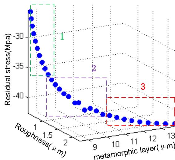
**Figure 4. Plastic Deformation Layer Thickness and Surface Roughness of Pareto Front**
