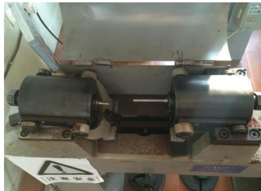
**Figure 3. Fatigue Test of Rotating Bending**
