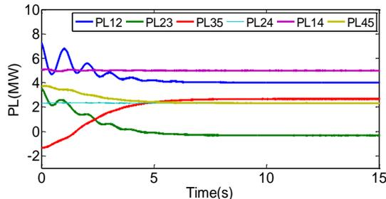
**Figure 10. Power flow with designed algorithm when Max-capacity Changes**
