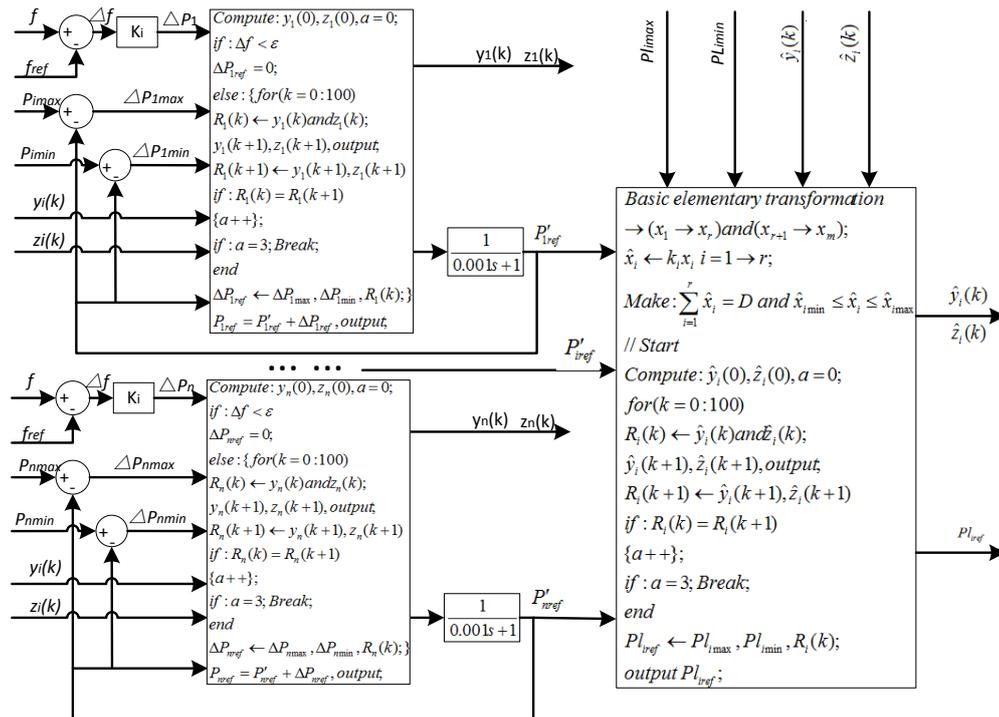
Figure 5. The Scheme of Frequency Regulation Controller
