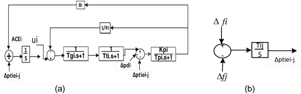
Figure 1. (a) Block Diagram of  $i^{\text{th}}$  Control Area. (b) Tie- Line Power
