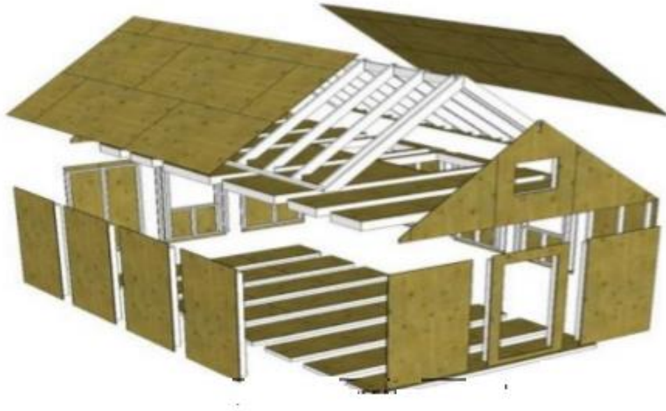
Figure 3. System of Prefabricated Construction
