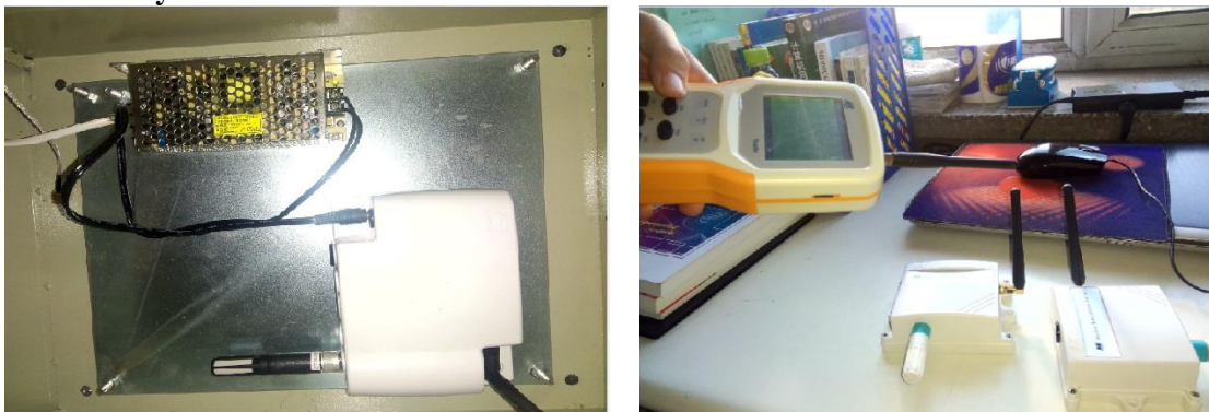
Figure 8. Temperature and Humidity Sensor and the Holding Collector
