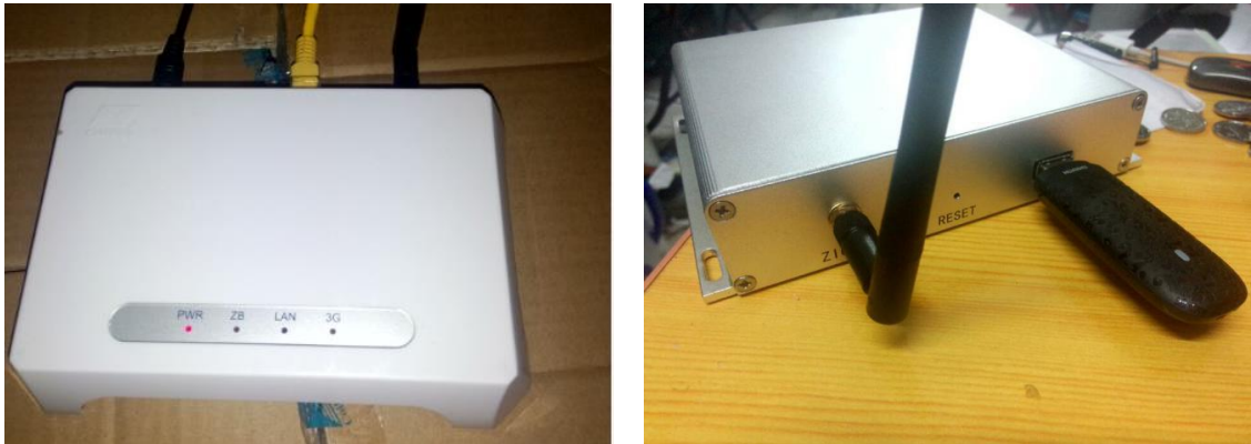
Figure 9. The Gateway Based on ZigBee Protocol and 3G Network
