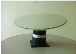
Figure 1. A Small Size Heliostat
