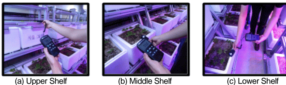
Figure 8. Illumination Measurement on Three Locations of Cultivation Shelves
