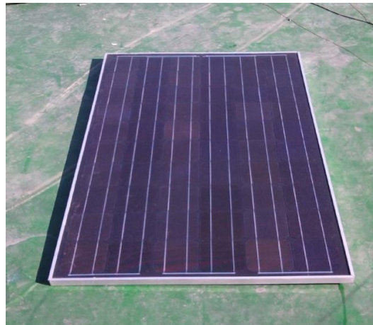
Figure 3. Macrograph of the Unglazed PVT Collector with a Rectangular Channel Absorber
