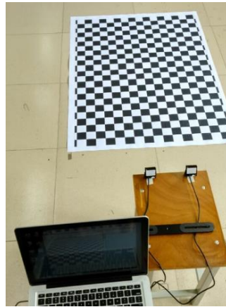
Figure 4. Binocular System Calibration in this Paper
