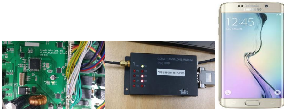
Figure 8. System of the Smart Applications: (a) MPU Board of the Receiver (b) CDMA Module (c) Smart Phone
