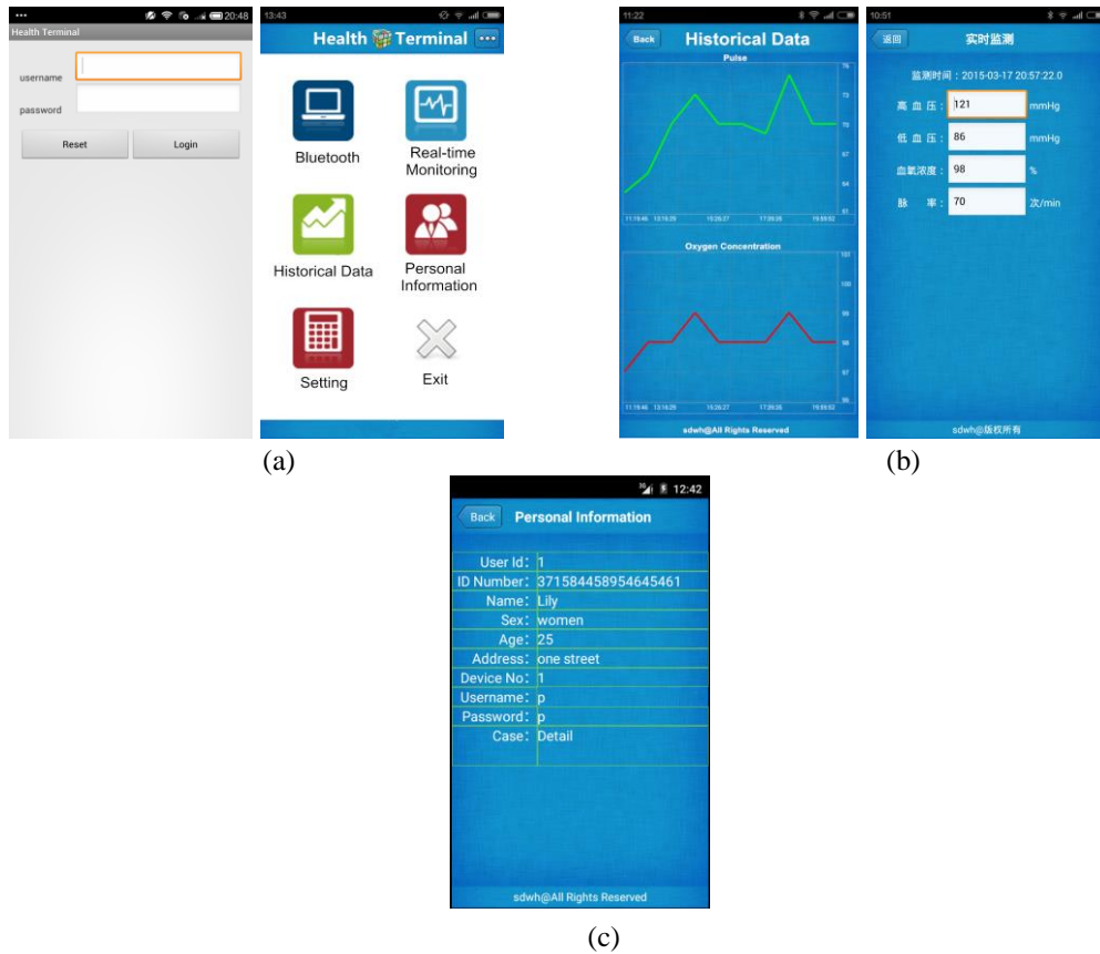
Figure 9. APP which is Designed for this System: (a)Android Login and Main Menu, (b) Historical Data Curve, (c) Real-time Monitoring and Personal Information
