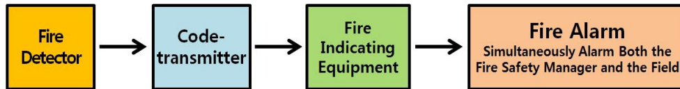
Figure 1. Block Diagram of the Current 4-Step Automatic Fire Detection System
