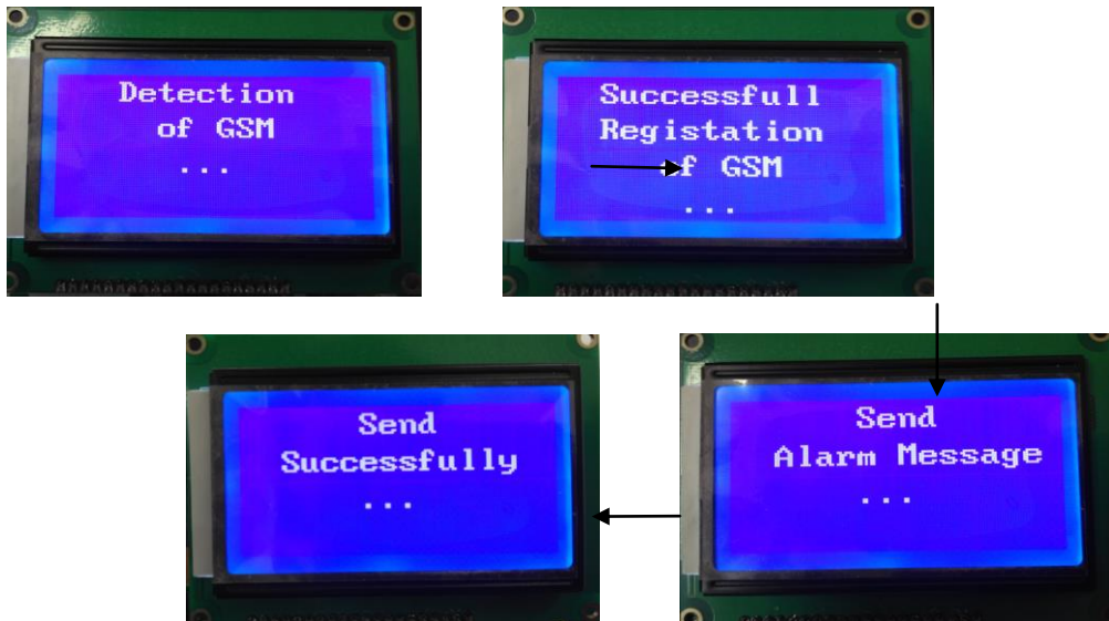
Figure 7. Transmission Process of Fire Alarm Short Message
