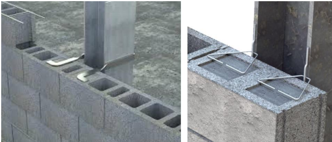
Figure 4. Tie-Down (Anchor Bolt) at VMT Site
